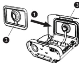
Confirm that the seal is positioned so the wire channel (2) in the seal is below the humidifier outlet port (3).
