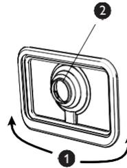
humidifier outlet port (2) until the center of the seal is fully seated. Finally, go back and run your fingers around the rectangular perimeter of the humidifier lid seal once more to confirm it has not become dislodged.
